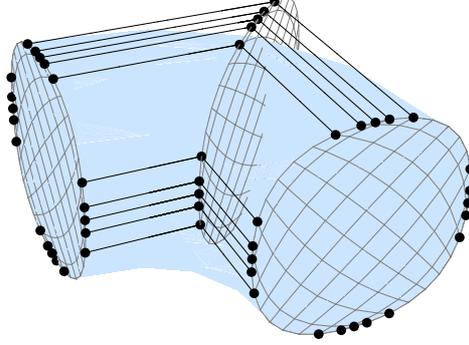
Figure 14: Quarter of a torus and control point grid
