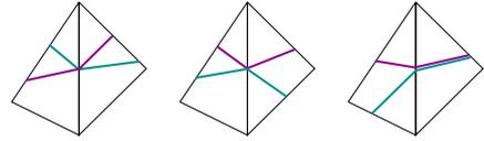
Figure 9: Piecewise linear level sets of  $f$  and  $g$  (colored) on boundary triangles (black) incident to the tested edge. Left: the usual case, level sets intersect. Middle: level sets touch without crossing, the edge in the middle is part of the Jacobi set. Right: needs special care, for example by reducing this case to a kind of lexicographic ordering. We will skip the technical details here.
