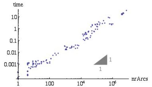
Figure 21: Computation time depending on total number of arcs in all level set Reeb graphs in a doubly logarithmic plot.
