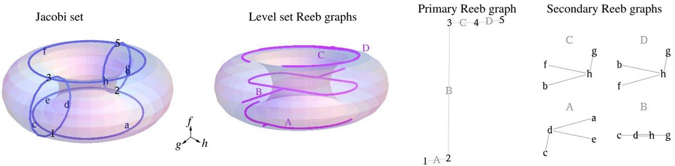
Figure 16: Example of a layered Reeb graph. In this example, the primary Reeb graph with respect to  $f$  contains only vertices of valency two. Event 4 is a swap event: In level set graph  $C$ , vertex  $f$  is slightly to the left of vertex  $b$ , and the two vertices are swapped in the transition to graph  $D$ .
