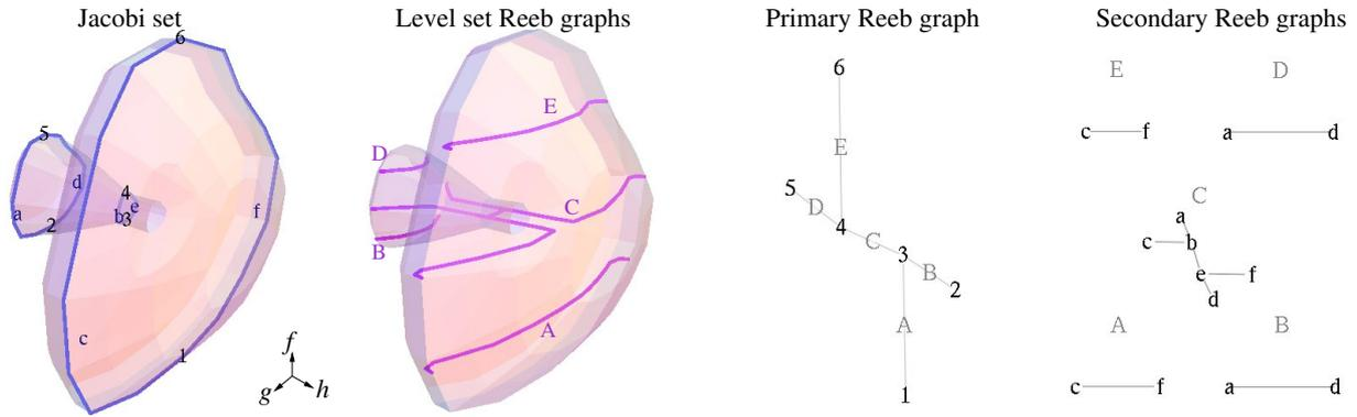
Figure 14: Example of a layered Reeb graph. Left: A mushroom-shaped object whose "cap" has a concave inner boundary. The blue lines show the Jacobi set. Center-left: Level set Reeb graphs embedded at the midpoints of the represented  $(f, g)$ -level sets. Center-right and right: Primary and secondary Reeb graphs. The graphs are drawn such that the  $f$ -value (or the  $g$ -value for the level set Reeb graphs) of a vertex serves as its  $y$  (or  $x$ ) coordinate in the planar picture.
