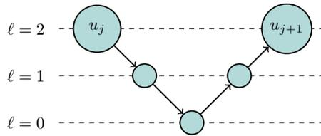
Figure 4: Visualization of one iteration of the multigrid V-cycle algorithm with three nested spaces. Circles correspond to smoothing operations or, on the coarsest level  $\ell = 0$ , the exact solve. Downward arrows correspond to restriction and upward arrows to prolongation operations.
