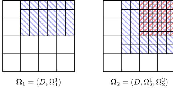
Figure 5: Two subdomain hierarchies over  $D = (0, 1)^2$  which satisfy (1) and (6). The subdomains  $\Omega_\ell^1$  are shown in blue, and  $\Omega_2^2$  is shown in red. Due to (1), each hierarchy  $\Omega_\ell$  induces a hierarchical spline space  $\mathcal{H}(\Omega_\ell)$  as defined in Section 2.1. Due to (6), the hierarchical spline spaces are nested,  $\mathcal{H}(\Omega_1) \subset \mathcal{H}(\Omega_2)$ .
