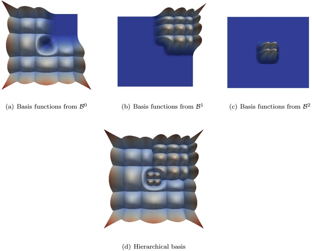
Figure 3: The contribution of basis functions from levels 0, 1 and 2 to the THB-splines  $\mathcal{T}$  defined over the subdomain structure shown in Figure 1. The effect of truncation is clearly visible in the central area of the domain.
