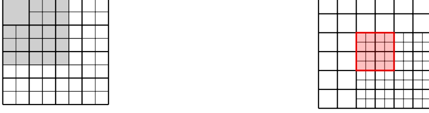
Figure 2: Left: Support of a cubic HB-spline (entire box) and of a THB-spline (grey) of level 0 on a hierarchy with two levels, N = 1 . The associated coefficient functional is supported on the larger cell (that belongs to \Omega^0 \setminus \Omega^1 ) in the top left corner. Right: Hierarchy of 2 levels \Omega^0 and \Omega^1 , subdomain \Delta = \hat{\Omega}^0 highlighted in red. We have \hat{\Omega}^0 = \Omega^1 , hence \hat{J}^0 = \emptyset and \hat{J}^1 \not\subseteq J^1 .
